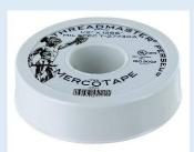
Totally maintenance free, Merco Threadmaster® Perseus™ is virtually chemically inert, non-toxic and non-flammable. Its 10 years shelf life\*\* allows prewrapping and storage of threaded parts. It will withstand temperatures from -450°F (-232°C) to 550°F (265°C), and pressures from a hard vacuum to 100 psi\*\*\*. This superior tape is made in an ISO 9002 certified
