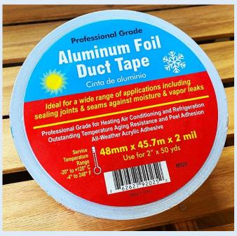
Merco M920 Aluminum Foil Tape is a 50 micron (2-mil) nominal dead soft aluminum foil with an aggressive cold weather solvent acrylic adhesive and protected by easy release liner.
