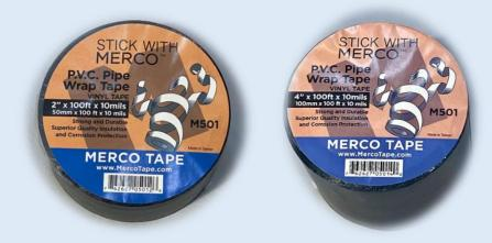
**Merco M501 series PVC Pipe Wrap Tape** is a 10-mil soft PVC tape intended for use as primary corrosion protection for under and above ground, metal and plastic pipe installations. It resists corrosion, moisture, bacteria, fungus and abrasion and is UV resistant.
