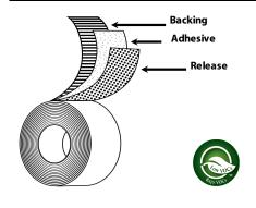
**Backing:** 2 mil Aluminum Foil - Printed
